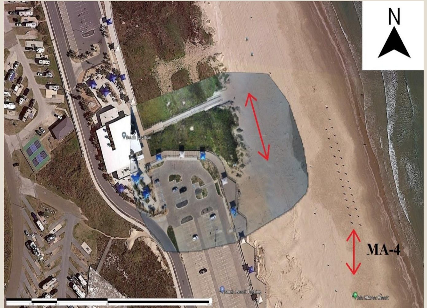
Figure 12: MA-4 orthomosaic generated with PIX4DMAPPER software using drone data
